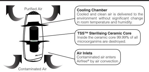
Regardless of how hazardous a virus, fungus or bacteria might be they are fully destroyed by the powerful heat inside the TSS™ ceramic core mini ducts. The heat inside the ceramic core forces sterilised air up to the heat exchanger causing air convection, which generates negative pressure underneath the ceramic core, so contaminated air is "sucked" in at Airfree® bottom air inlets in a continuous, silent, and efficient air flow.
